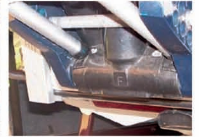
Evinrude 'indent' location - place round ends UNDER the pin and into 'indent' features.
